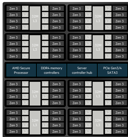
FIGURE 4. AMD EPYC 7003 Series processor high-level processor design 6
